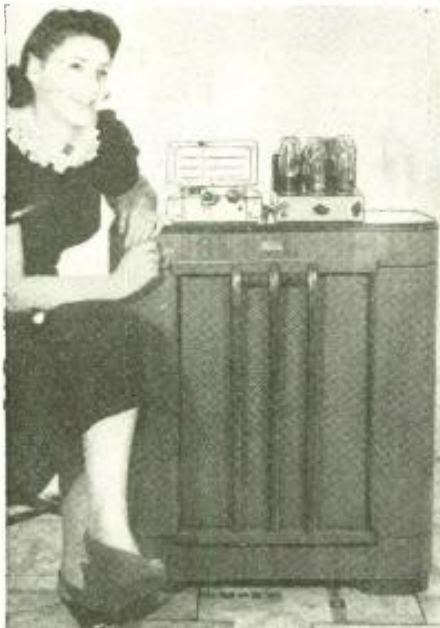
The high-fidelity Jensen loudspeaker and its cabinet is shown in the picture, together with the F-M tuner and audio amplifier on top of it.
