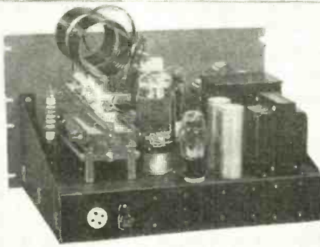
Right—The complete 750 watt transmitter fits into this 28" Par-Metal rack. Note the crystal which plugs directly into the front panel.
