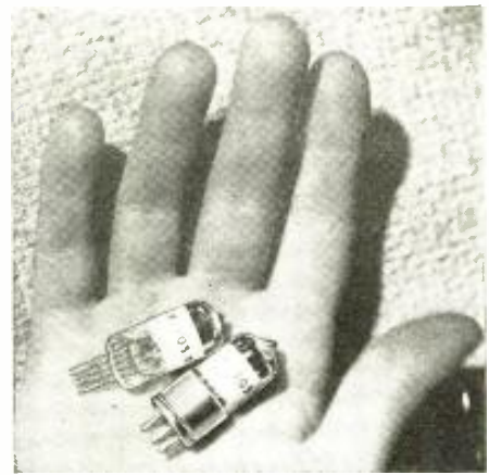
Note the extremely small size of the new Raytheon pentode amplifiers.
