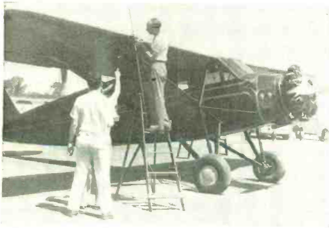
Fitting the antenna for the 112-mc. transmitter and receiver onto the airplane used in the tests.
